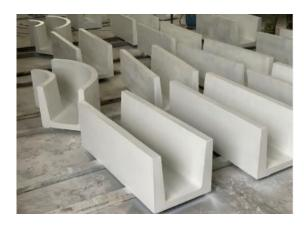
The aluminum free castable preform solves the problem of reaction between refractory materials used in aluminum industry and molten aluminum. The new composite castable prepared by ourselves will not produce aluminum ash, corrode, nodulate and adhere to aluminum in the process of molten aluminum smelting, which can greatly reduce the loss of molten aluminum in the process of aluminum smelting.
